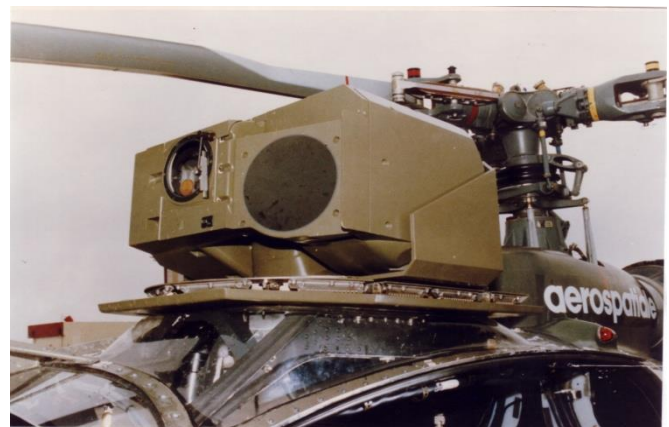
INSTRUMENT MODULE BELOW THE HEAD ROTOR OF A HELICOPTER – WIRE ROPE ISOLATOR (SOCITEC-)
